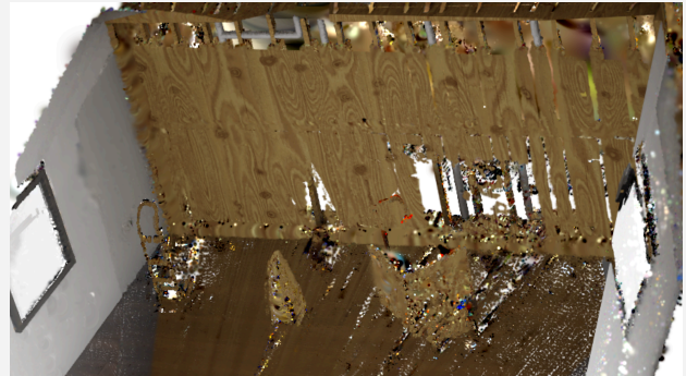
Figure 6: The “Paint-Over” Effect The same scene in Fig. 3 from a different perspective to show the geometric errors.
